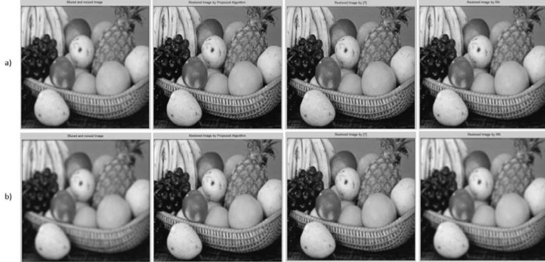
Fig. 2. Restored fruit images by proposed method and reduced Newton: a) Noise Variance = 2, Sigma = 4.4, r = 5 and b) Noise Variance = 2.5, Sigma = 8.4, r = 7.
